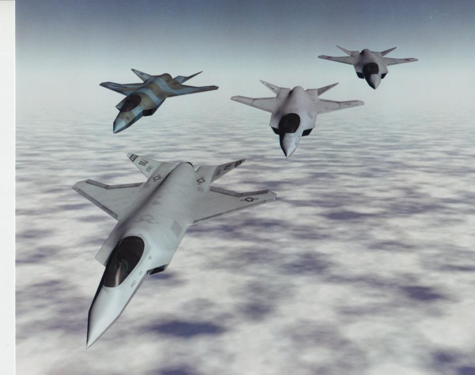
Pictured here are the three variants of the McDonnell Douglas, Northrop Grumman and British Aerospace entry in the Joint Strike Fighter (JSF) competition. The JSF will be an affordable family of strike fighters that meets the requirements of the U.S. Air Force, the U.S. Navy, the U.S. Marine Corps and the U.K. Royal Navy. This stealthy aircraft's vertical tails have been removed, and an innovative engine thrust-vectoring nozzle is used to manoeuver the aircraft.
