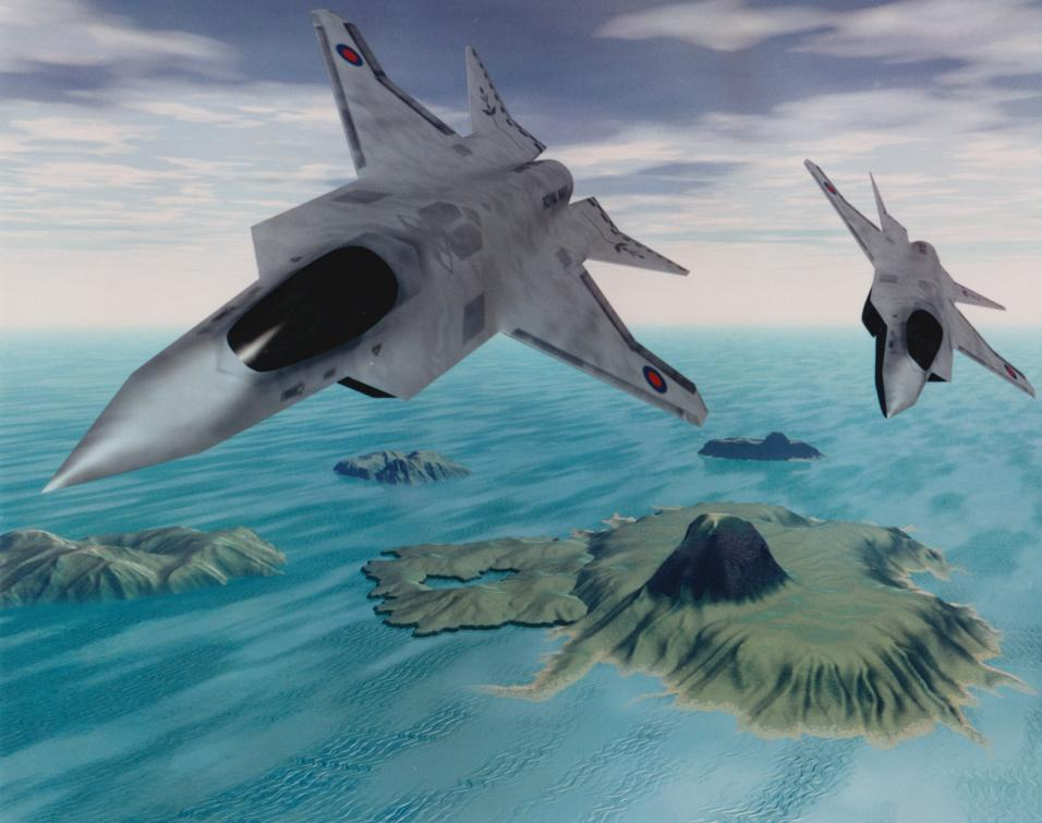
The Royal Navy is looking at the Joint Strike Fighter (JSF) as a replacement for the Sea Harrier. Designed for stealth, the JSF's vertical tails have been removed, and aninnovative engine thrust-vectoring nozzleis used to manoeuver the aircraft. The JSFwill be an affordable family of strikefighters for the U.S Air Force, the U.S Navy, the U.S. Marine Corps and the U.K. Royal Navy.
