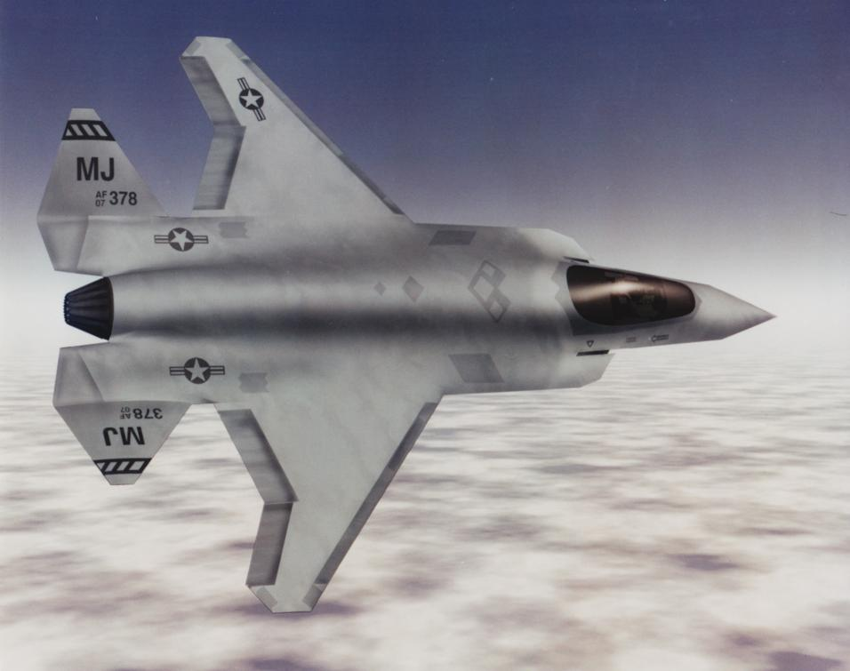
This is the Air Force version of the McDonnell Douglas, Northrop Grumman and British Aerospace entry in the Joint Strike Fighter competition. Removing the vertical tails and use of an innovative engine thrust-vectoring nozzle results in an aircraft that is virtually spin proof.
