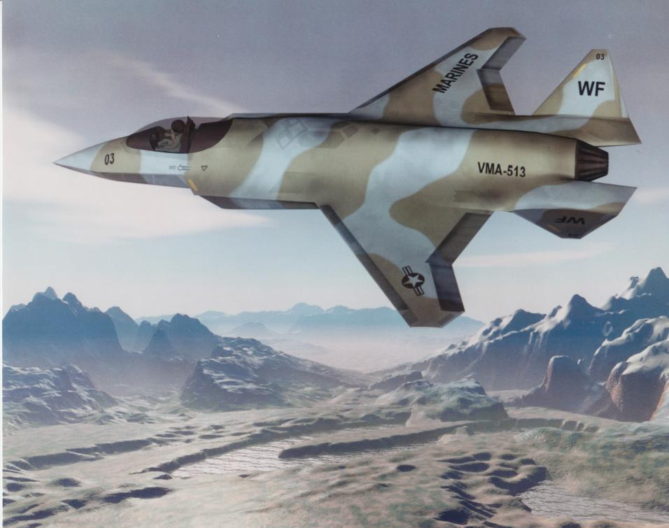
The Marine version of the McDonnell Douglas, Northrop Grumman and British Aerospace entry in the Joint Strike Fighter competition has a forward lift engine in addition to the main cruise engine. Designed for stealth, the aircraft's vertical tails have been removed, and an innovative engine thrust-vectoring nozzle is used to manoeuver the aircraft.
